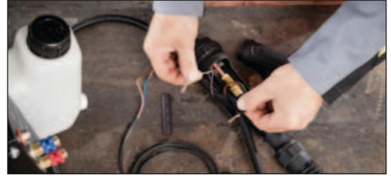
2. Disassemble end of the trigger cable.
